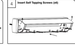
Now insert x6 appropriate length self tapping screws (not supplied) into the remaining holes to fix the letterplate securely to the door.
